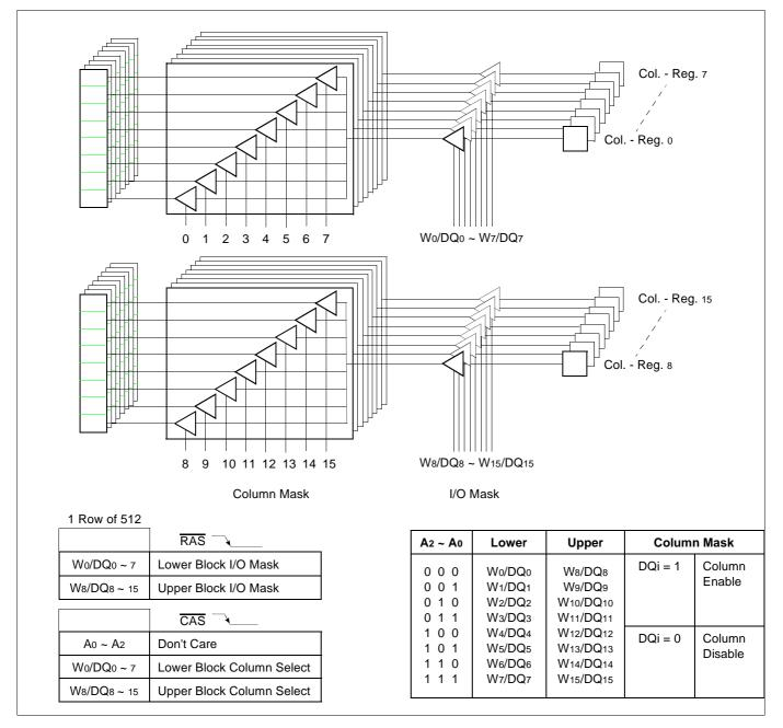
Figure 5. Block Write Scheme
