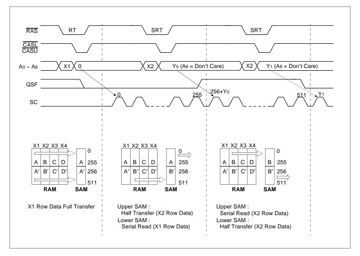
Figure 7. Split Read Transfer Normal Usage
