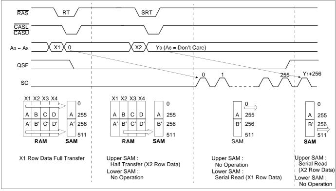
Figure 8. Split Read Transfer Normal Usage
